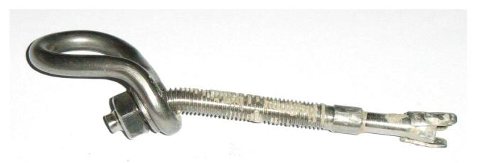
*The second bolt pulled out with loads varying between 3.5kN and 10kN, nearly losing the clip on the way.*
