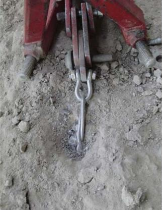
39kN on a radial pull, the rock has collapsed to about 5cm depth and now a pebble is taking the strain, luck of the draw. This bolt went on to hold 45.2kN
