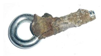
This one was not very impressive (Hilti eyebolt) in the radial tests coming out covered in sandy rubble at 11kN, as one can see drilling an accurate hole is difficult. The only bit that really held is the grey area down the bottom!
